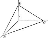
Scholium 5. If the plane is perpendicular to the plane YX, its trace CD, will be parallel to the axis of Z: and hence, the tangent of the angle which it makes with Z will be 0: this will give
